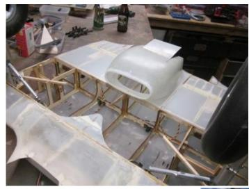
skin under stress as the bottom section is open for the wheel wells.
