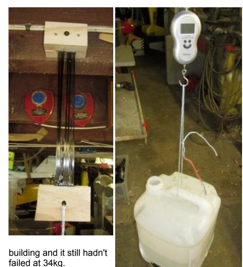
blocks, screwed one end to the rafters and applied weights to the other end with a fish scale in between.
