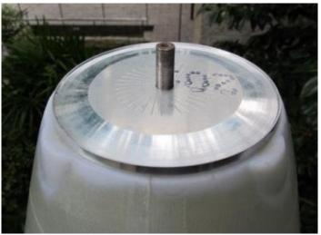
I hung the fuselage over the edge of our deck again and centred the engine with the cowl and spinner backplate in position, removed backplate and cowl, marked engine position on mounting plate, drilled and bolted into position. The best part of all this is that it still all fits inside the cowl.
