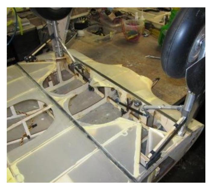
I'm now fairly confident that I have added about 100kg of strength across the structure by laminating two tows on the front beam and one on the rear beam. I've laminated the tows with strips of 2oz. glass to bond them to the spars and fair them into the surface.
