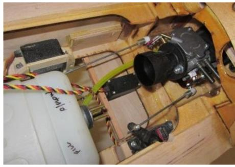
The picture on the left is of the throttle servo, Hitec HS635HB rated at 6 Kg/cm and the Hextronic HX5010 7kg choke servo,
